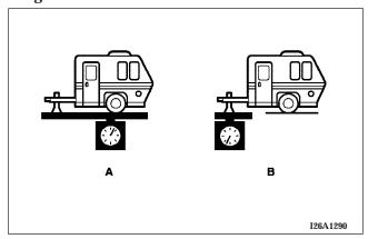
Never exceed the maximum trailer weight (A), maximum tongue weight (B), Gross Vehicle Weight Rating (GVWR) and Gross Axle Weight Rating (GAWR).
